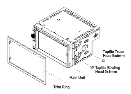
TYPICAL FRONT-LOAD DIN MOUNTING METHOD
