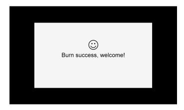
6. Remove the USB stick , Power off then Power on the receiver. Once the receiver reboots, this will conform the 1st update was done successfully.
