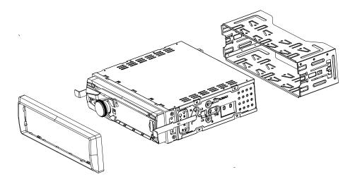
TYPICAL FRONT-LOAD DIN MOUNTING METHOD
