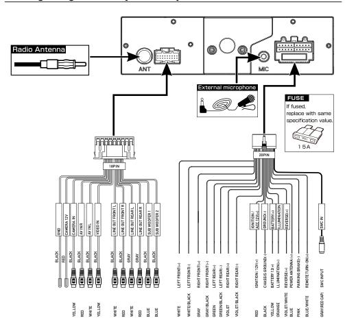
When replacing a fuse, make sure to use the correct type and amperage. Using an incorrect fuse could cause damage. The unit uses (1) 15 amp ATC mini style fuse located on the power connector
