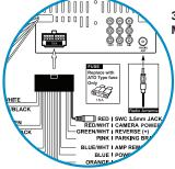
3.5mm SWC port located on the rear of the unit, on the MAIN POWER I/O Harness
