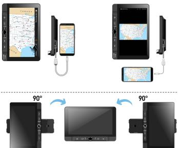
Tip: Manually rotate the monitor to the left or right until locked in the horizontal position.
