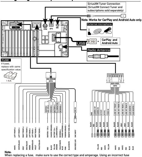
could cause damage. The unit uses (1) 15 amp ATC mini style fuse located on the power connector
