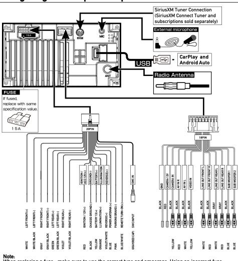
Note: When replacing a fuse, make sure to use the correct type and amperage. Using an incorrect fuse could cause damage. The unit uses (1) 15 amp ATC mini style fuse located on the power connector.
