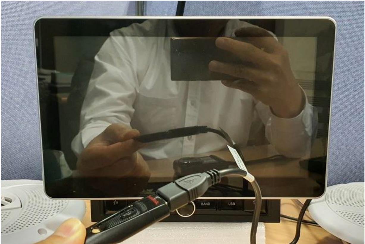
10. After ACC Power On, after a while, the following Bar is displayed and the firmware update is performed.
