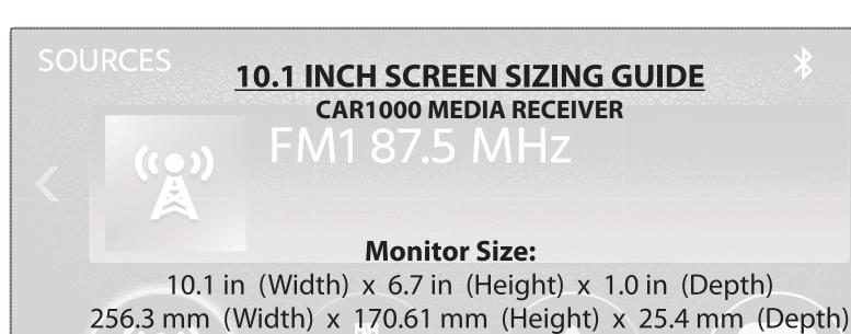
Cut along the dotted line to use this as template for gauging if the CAR1000 receiver will fit in your car
