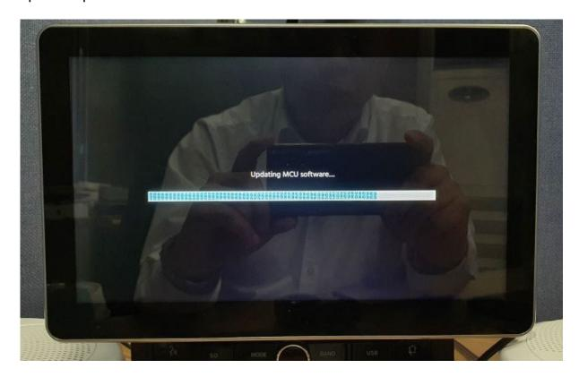
11. When MCU Firmware Update is completed and displayed on the screen as shown below, press the OK Icon. In 10 seconds, you can remove the USB Thumb Drive from the unit.
