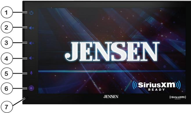
**Power On/Off** ① Press any button to turn the unit on. Press **POWER** and hold to turn the unit off.
