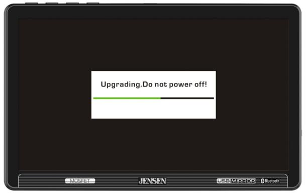
7. Once the update is complete you will see the below screen. Remove the USB thumb drive and turn your vehicle off and then back on. This will complete the 1<sup>st</sup> part of the update.
