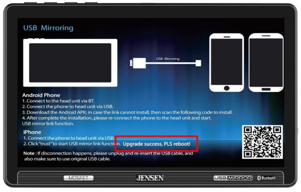
7. After turning the ignition off and then back on, switch to the USB Mirroring Mode of the receiver to check that the update was successful. The below image shows the updated software version of the updated firmware.
