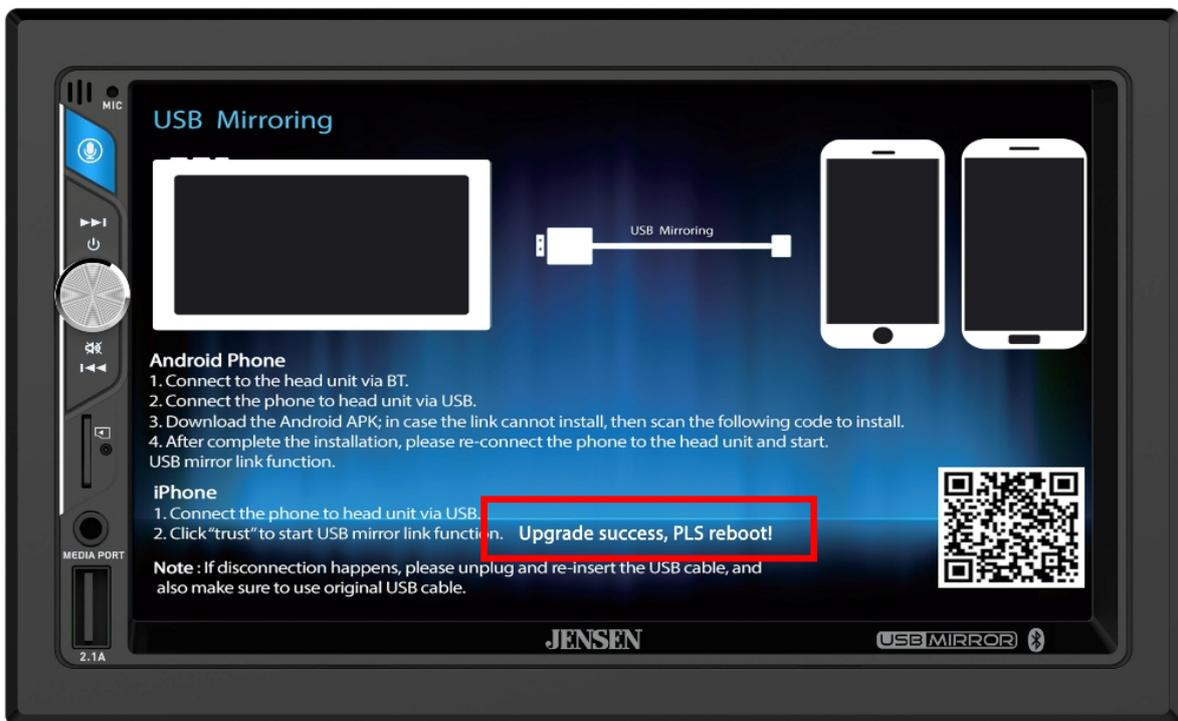
7. After turning the ignition off and then back on, switch to the USB Mirroring Mode of the receiver to check that the update was successful. The below image shows the updated software version of the updated firmware.
