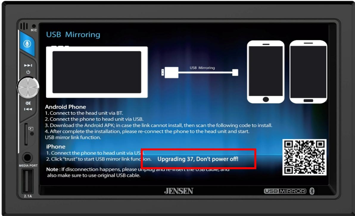
6. Once the update has completed, you will see the below screen. Remove the USB thumb drive and turn your vehicle off and then back on to reboot the receiver.
