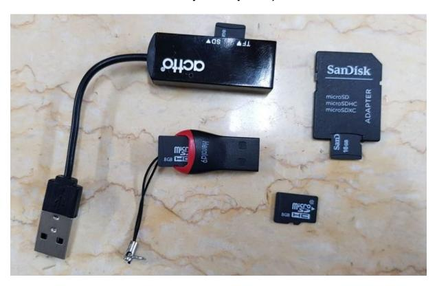
Plug the microSD card adapter or USB/microSD card reader into a USB port of your computer. Copy all files contained in the firmware folder on your desktop onto the blank microSD card. DO NOT PUT ANY FILES INTO ANY FOLDER, ALL FILES SHOULD BE ON THE ROOT OF THE SD CARD.
