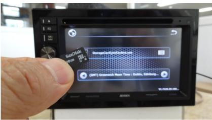
Next, go to the Settings from the Main Menu screen and tab over till you get to the Version page. Press the Version tab and the Reset Nav pop-up window will appear on the screen. Next, press Ok on the screen to return to the Navigation screen.
