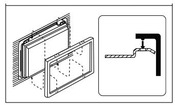
NOTE: For proper operation of the CD/DVD player, the chassis must be mounted within 30° of horizontal. Make sure the unit is mounted within this limitation.
