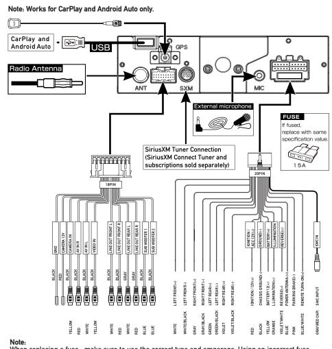
When replacing a fuse, make sure to use the correct type and amperage. Using an incorrect fuse could cause damage. The unit uses (1) 15 amp ATC mini style fuse located on the power connector. Wiring Notes:
