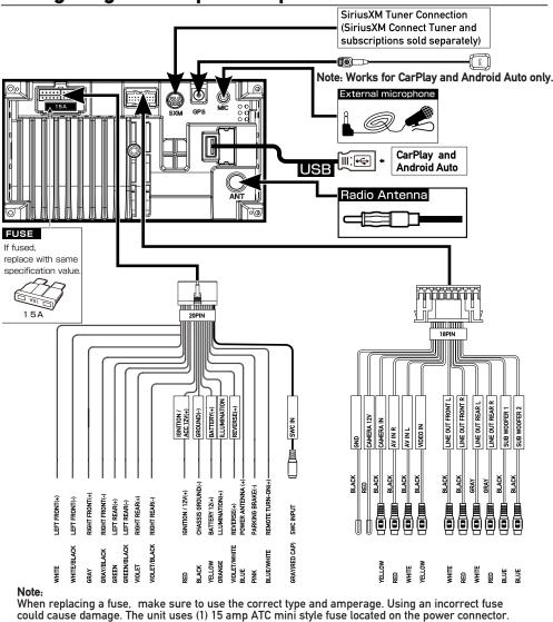
Wiring Notes: Subwoofer output The Subwoofer preamp audio output (Blue jacket with Black RCA) is active in all audio modes.
