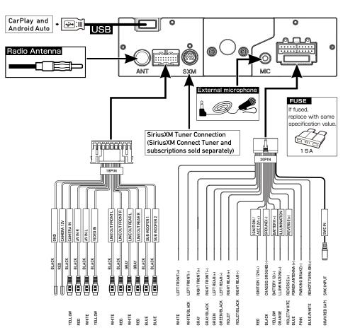
When replacing a fuse, make sure to use the correct type and amperage. Using an incorrect fuse could cause damage. The unit uses (1) 15 amp ATC mini style fuse located on the power connector
