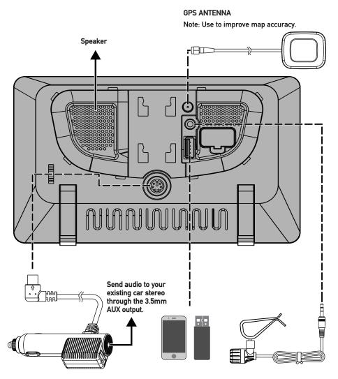
12V Power Adapter USB port for charging only (2.1A) 3.5mm output to connect audio to your car stereo
