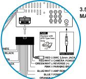
3.5mm SWC port located on the rear of the unit, on the MAIN POWER I/O Harness
